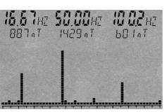
LF spectrum display and automatic multi-marker display on the digital screen of SPECTRAN® (Screenshot)
