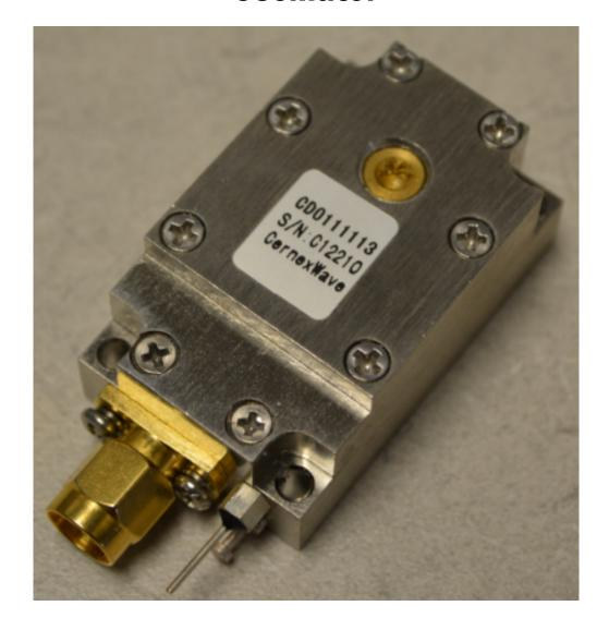
Cernexwave's CDO Series Dielectric Resonator Oscillators are offered in frequencies from 2 to 30GHz with outputs as high as 27dBm. They have low phase noise, excellent stability and the harmonics and spurious signals are limited.
