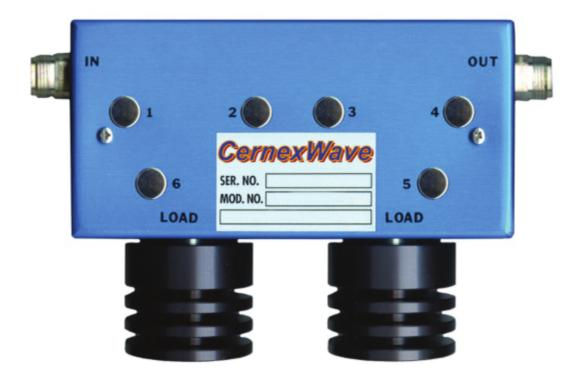
Cernexwave's Low Frequency Precision Dual Junction Isolators can can be tuned to any operating frequency from 66-108MHz. These devices are perfect for systems that require very high isolation with a minimum of insertion loss and VSWR. They can support 50W of average power forward and even more in reverse to protect sensitive devices from errant signals.
