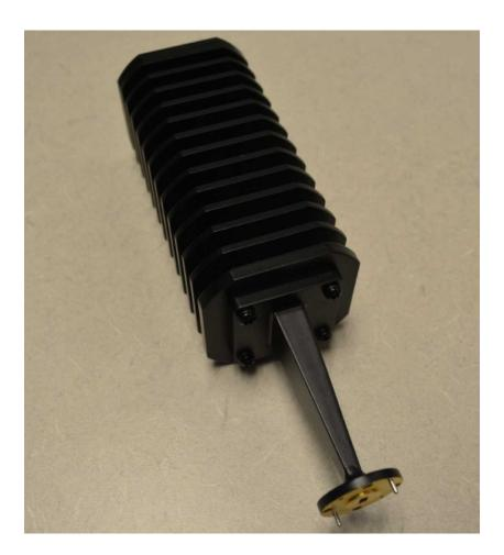
Cernexwave's Broad Band High-Power Air-Cooled Loads are made in waveguide sizes from WR-10 to WR-430 with power ratings anywhere from 1 Watt to 2500 Watts. They are designed so that virtually all of the applied power is absorbed assuring a low VSWR.
