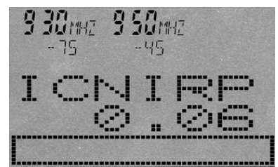
SPECTRAN® displays exposure limits both as percentage as well as a bargraph display. Our example shows approximation to the ICNIRP exposure limits by 0,06%. (Screenshot)
